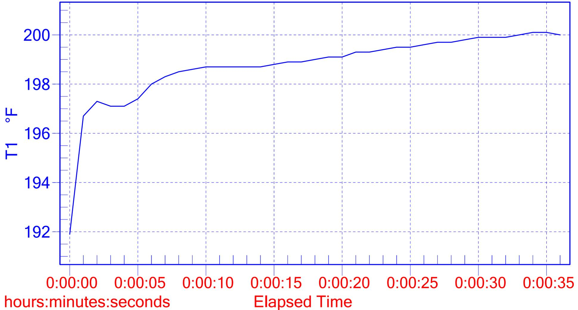
Dream 94C, +6C Offset. 2nd run. Removed PF for about 20 seconds to allow reheat and approx time if coffee has been ground and tamped. All readings auto-shutoff after 2oz dispensed. Note this is converted to Fahrenheit by the graphing SW. It should compare to 201F and +10.8F offset
