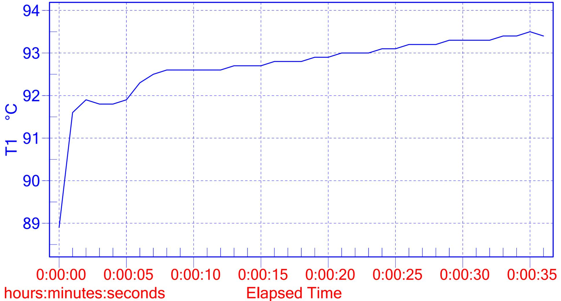
Dream 94C, +6C Offset. 2nd run. removed PF for about 20 seconds to allow reheat and approx time if coffe has been ground and tamped. All readings auto-shutoff after 2oz dispensed.
