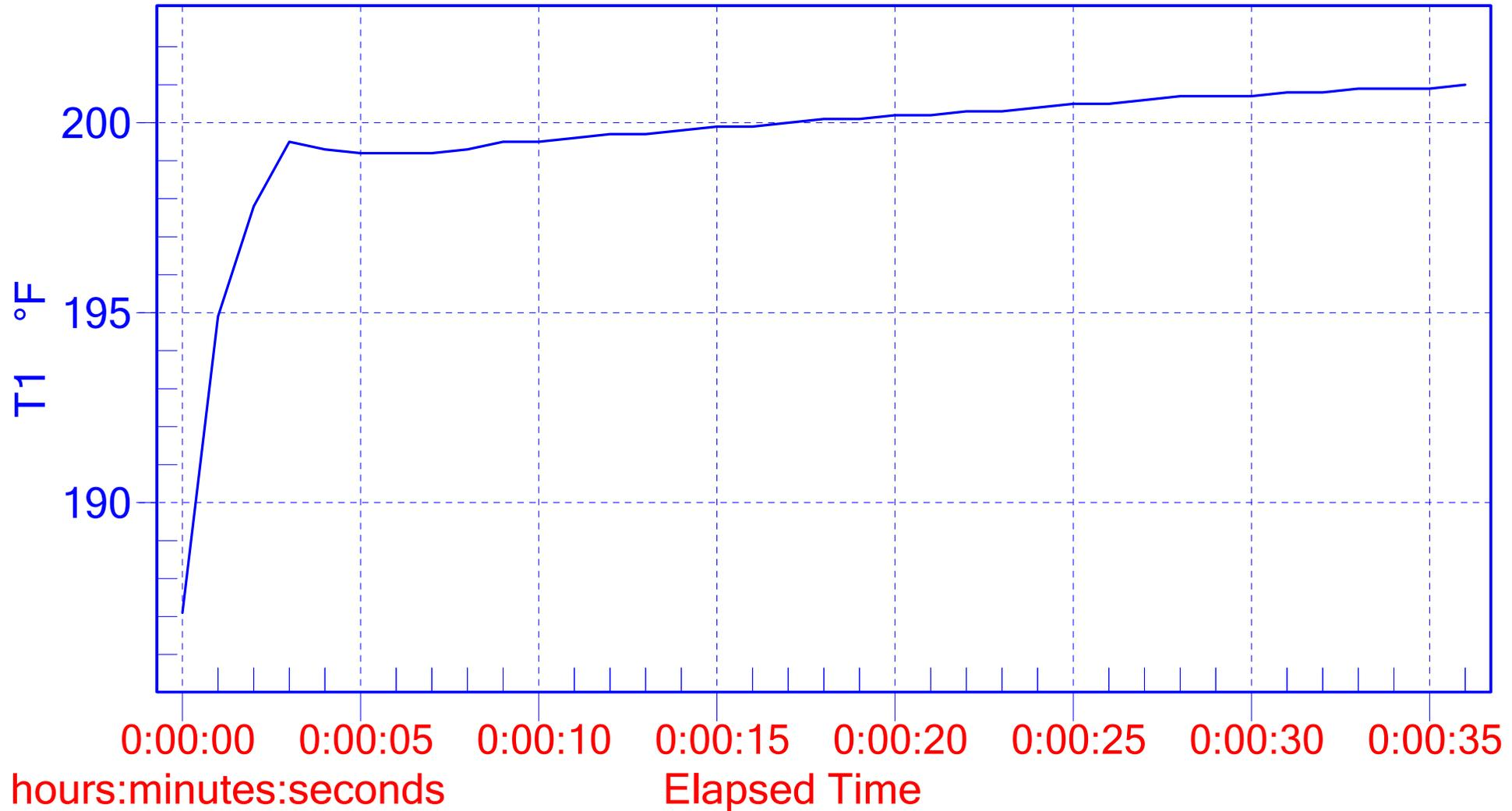
Dream 94C, +6C Offset. 4th run. removed PF for about 20 seconds to allow reheat and approx time if coffe has been ground and tamped. All readings auto-shutoff after 2oz dispensed. Fahrenheit conversion performed by meter SW. No changes made to Dream settings.
