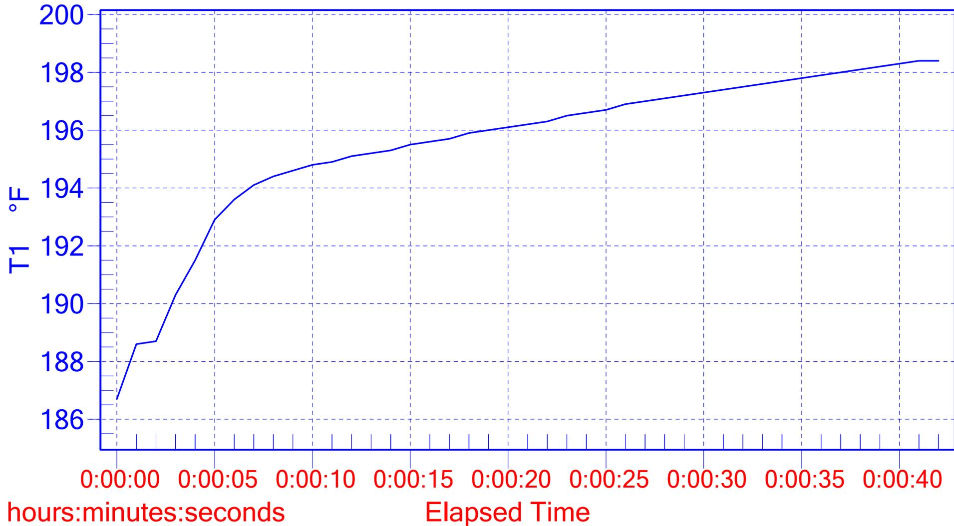
Dream Run 1 after about 1 hour idle time. 94C and +6 offset. Automatic run time for 2oz volumetric dose.
