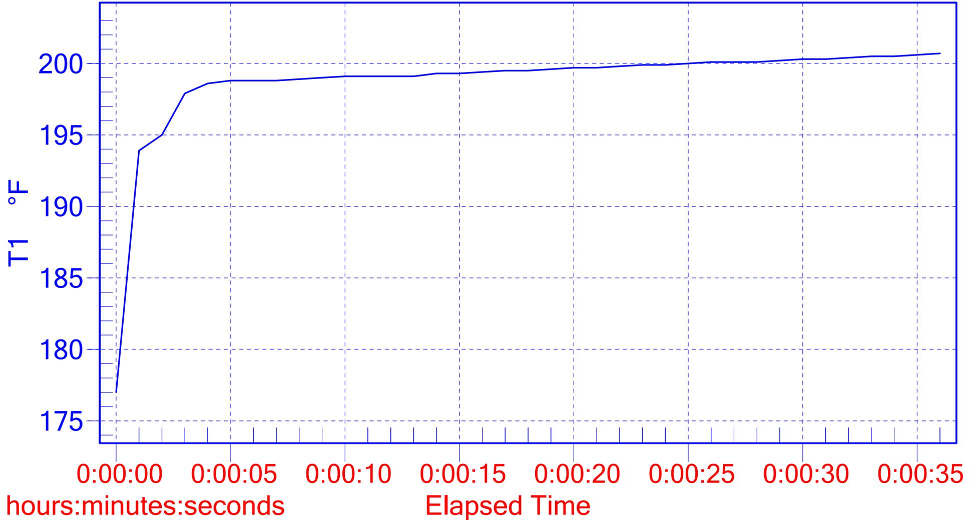
Dream 94C, +6C Offset. 3rd run. removed PF for about 20 seconds to allow reheat and approx time if coffe has been ground and tamped. All readings auto-shutoff after 2oz dispensed. Farenheit conversion is by meter SW. No changes made in machine settings.
