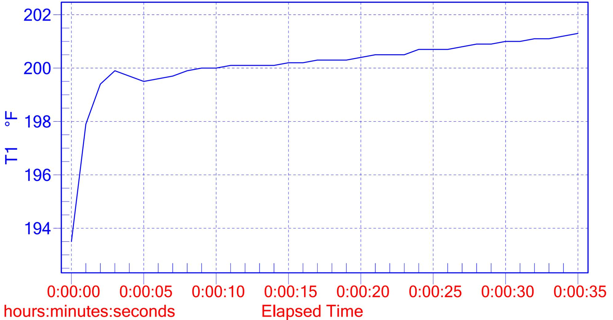
Dream 94C, +6C Offset. 5th run. removed PF for about 20 seconds to allow reheat and approx time if coffe has been ground and tamped. All readings auto-shutoff after 2oz dispensed. Fahrenheit conversion performed by meter SW. No changes made to Dream settings.
