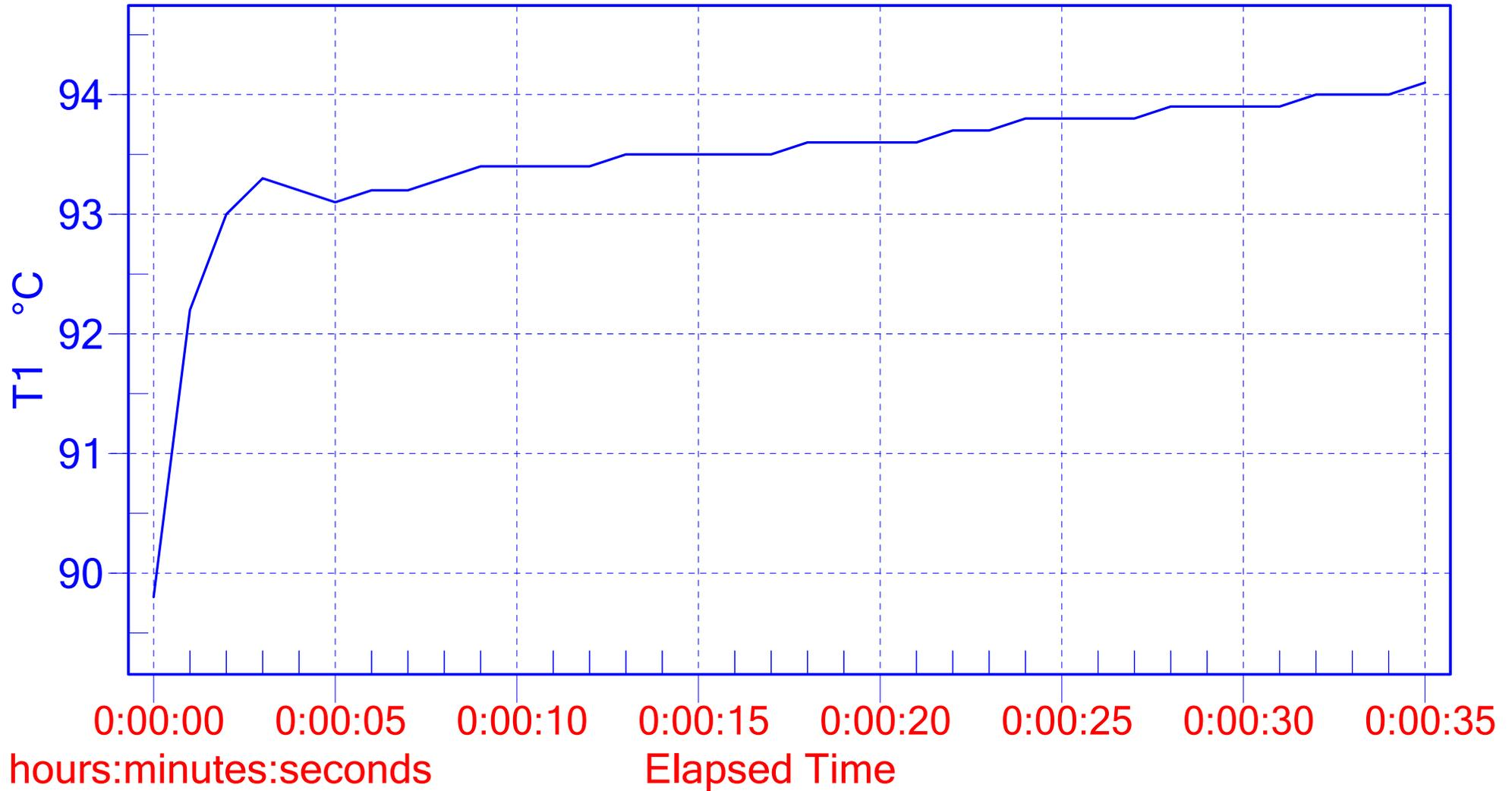
Dream 94C, +6C Offset. 5th run. removed PF for about 20 seconds to allow reheat and approx time if coffe has been ground and tamped. All readings auto-shutoff after 2oz dispensed.
