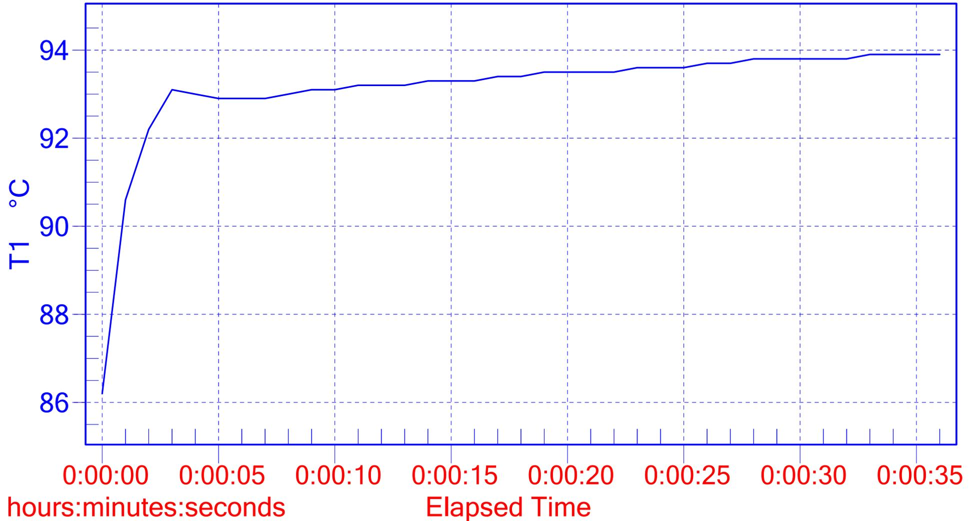
Dream 94C, +6C Offset. 4th run. removed PF for about 20 seconds to allow reheat and approx time if coffe has been ground and tamped. All readings auto-shutoff after 2oz dispensed.
