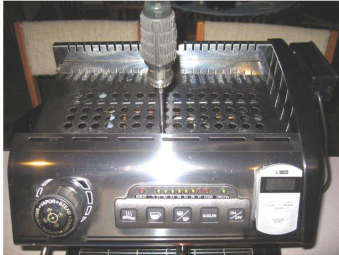
4. From the front of the machine look down into the top of the machine. In the right rear of the machine you will see a toggle switch with its positions labeled 15 and 20. Reach down with the same screwdriver you used to remove the cup warming tray and flip the switch to the desired position.
