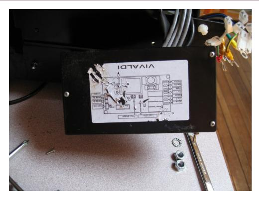
• Now you can see that there are another 8 cables passing through a slot in the side of the case that need to be dealt with. Remove the three screws shown in the above photo and pull the cover off the controller box.
