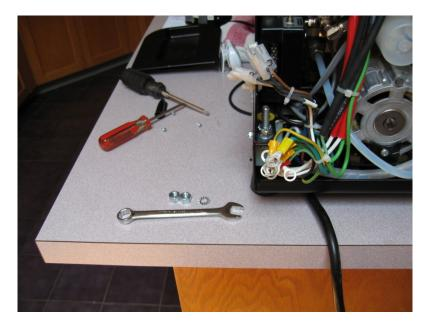
• The next step requires that you unscrew the three silver Phillips screws holding the black plastic controller box to the right side of the chassis.
